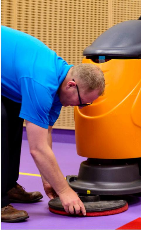
Attach the red pad underneath the scrubbing/suction machine.
