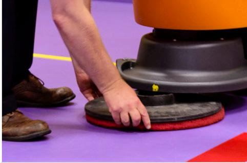
Attach the red pad underneath the scrubbing/suction machine.
